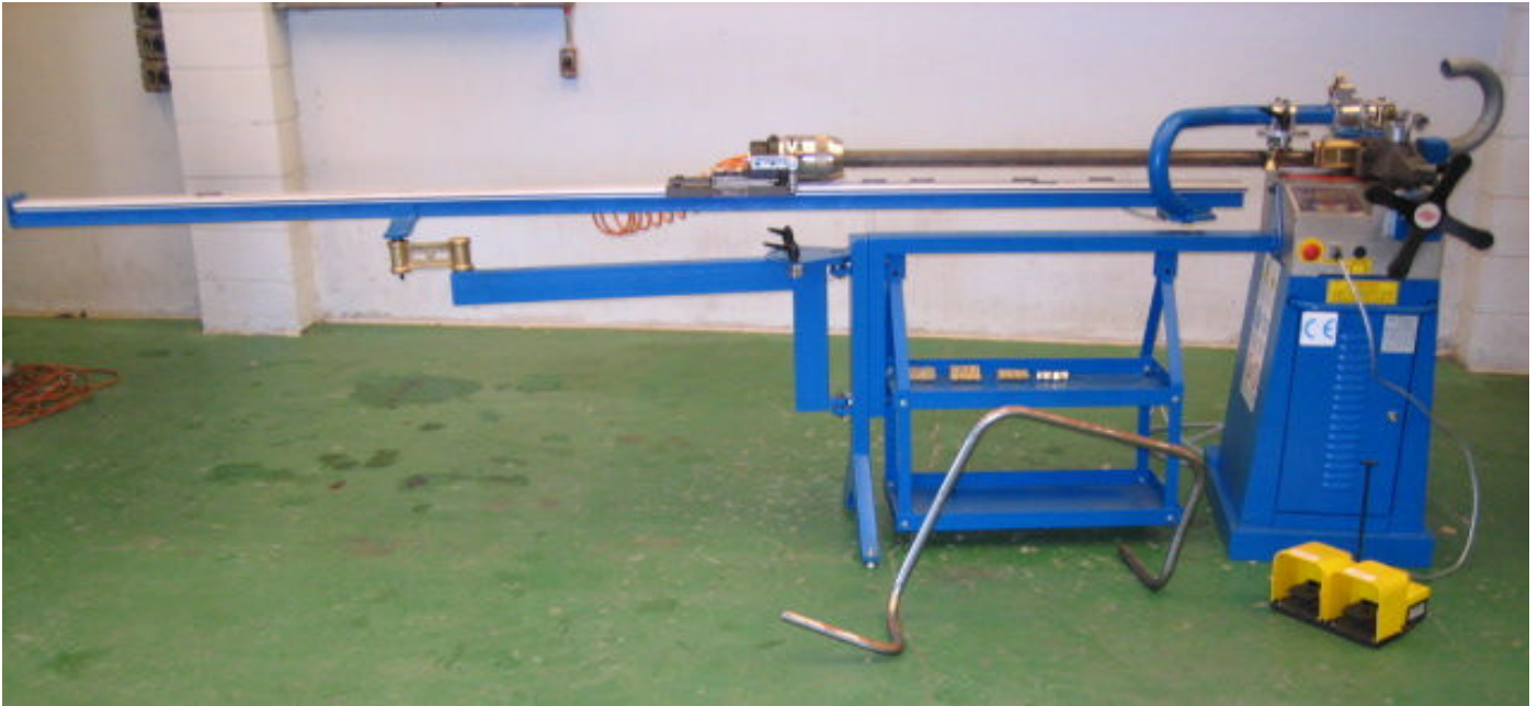
Photo showing model TB 050 with option 2 Axis positioning device
